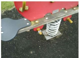
Finding: The end of handgrips and/or footrests have a cross section of less than 15cm2 and fail to meet the requirements of BS EN 1176:2008
