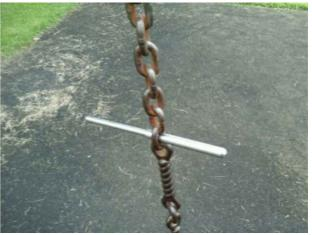
The chain openings are in excess of the 8.6mm as recommended by BS EN 1176
