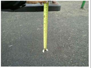
Finding: The seat clearance from finished surface level to the underside of the seat is too low.
